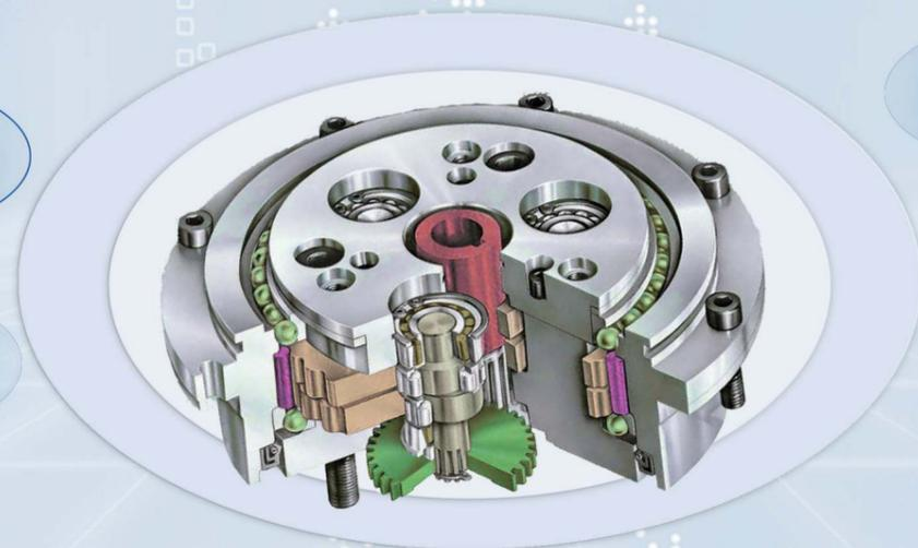
Low noise internal helical gear design
