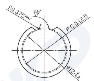
Detailed drawing of spline section
