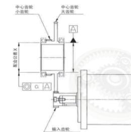
(Unit/mm) Specifications of small center gear tooth
