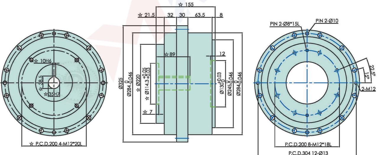
1. "★"The dimensions modify with motor specification.
