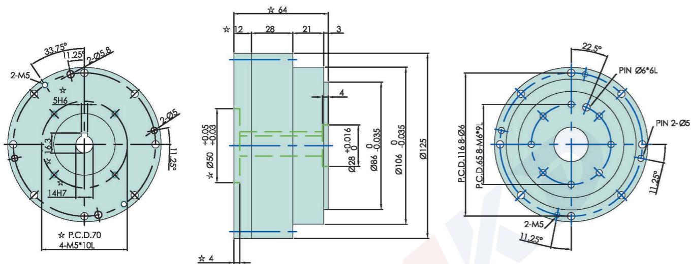
1. "★"The dimensions modify with motor specification.
