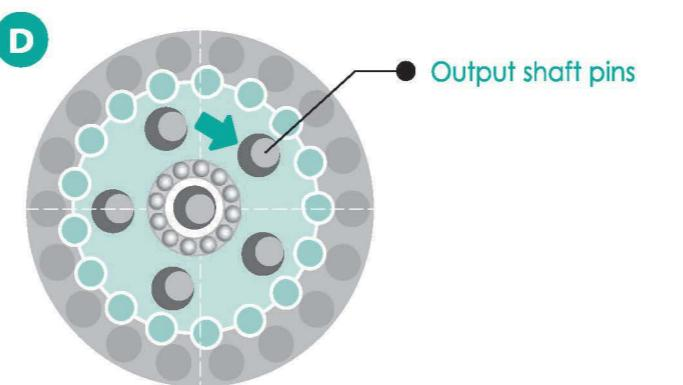
6.While internal rollers turning counter-clockwise accompanied with roller disc,this make rotationof internal rollers and external rollers separatelyfollow individual center axis due to mesh transmission.
