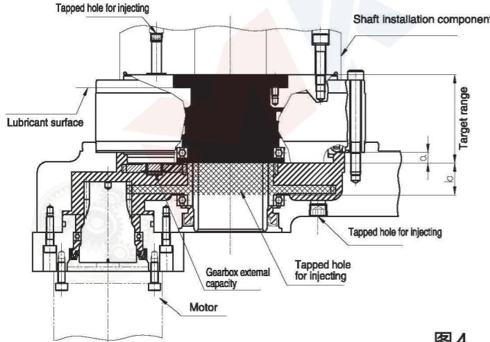
Vertical shaft installation (with shaft facing downward)
