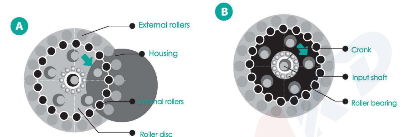
1. Cylindrical external rollers mounted in robust housing.
