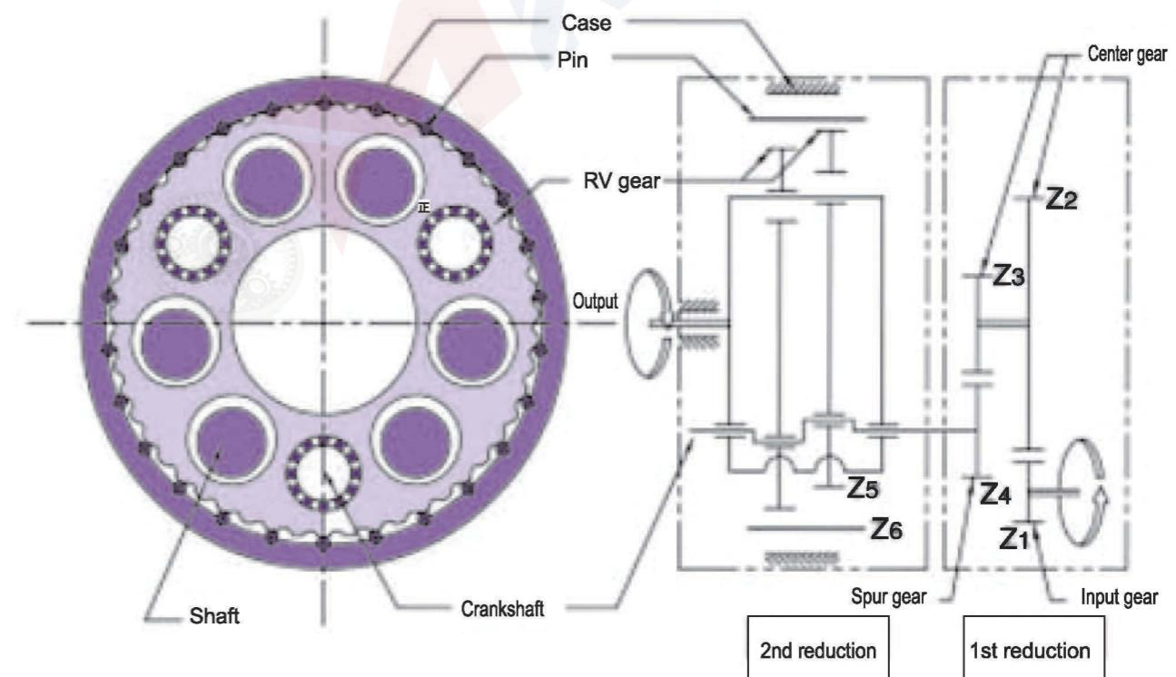
The overall reduction ratio  $i$  (of the First and Second reduction stages) will differ depending on the use, and can be calculated using the speed ratio values displayed in the table below.
