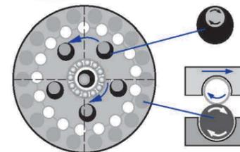
▲ Drive of external & internal rollers involved sliding and rotation-self, obtain extremely high efficiency.
