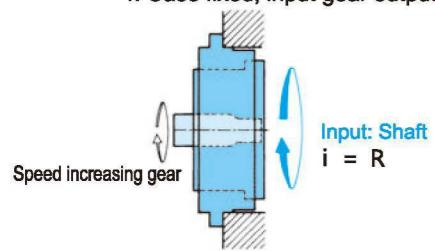
5. Shaft fixed, input gear output
