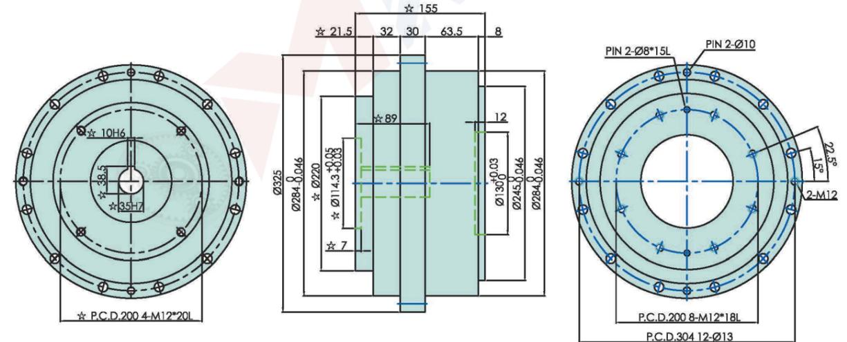
1. "☆"The dimensions modify with motor specification.
