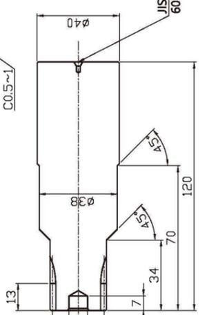
Input spline (standard) enlarged drawing
