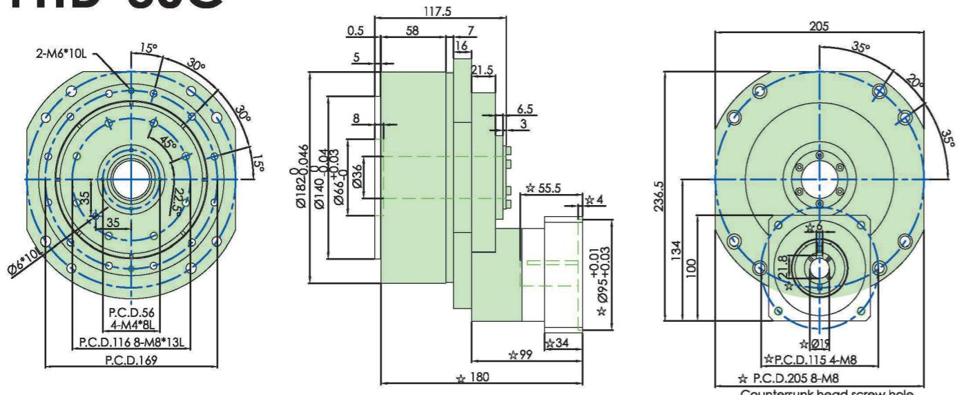
1. "★"The dimensions modify with motor specification.
