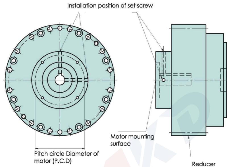
1. Place motor shaft key and reducer input shaft key way in a straight line, and insert motor shaft into reducer input shaft.
