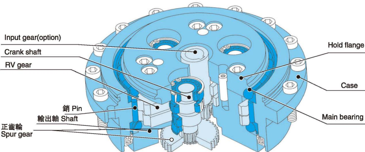
**Integrated angular ball bearings**
