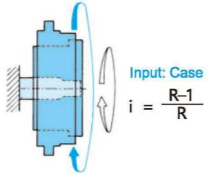
4. Case fixed, input gear output
