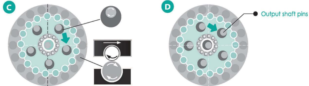
6.While internal rollers turning counter-clockwise accompanied with roller disc,this make rotation of internal rollers and external rollers separately follow individual center axis due to mesh transmission.
