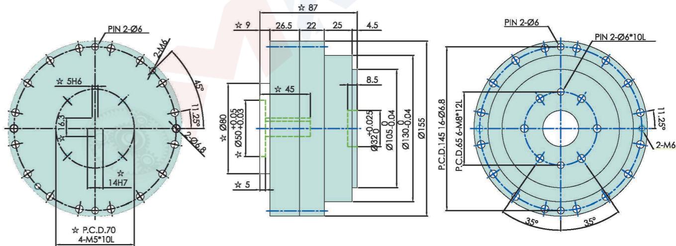
1. "☆"The dimensions modify with motor specification.
