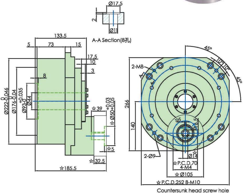
1. "☆"The dimensions modify with motor specification.
