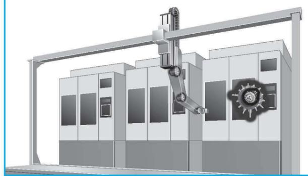
Machine tool ATC tool magazine
