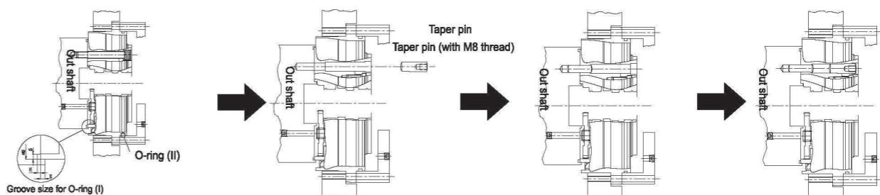
1. Loosely tighten the hexagon socket head cap screw to temporarily secure the gearbox shaft to the output shaft.
