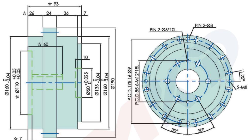
1. "☆"The dimensions modify with motor specification.
