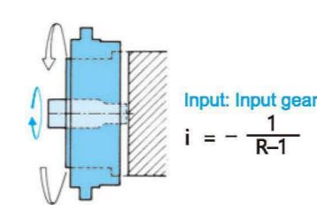
3. Input gear fixed, shaft output
