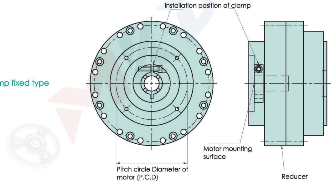
1. Place motor shaft key and reducer input shaft key way in a straight line, and insert motor shaft into reducer input shaft.
