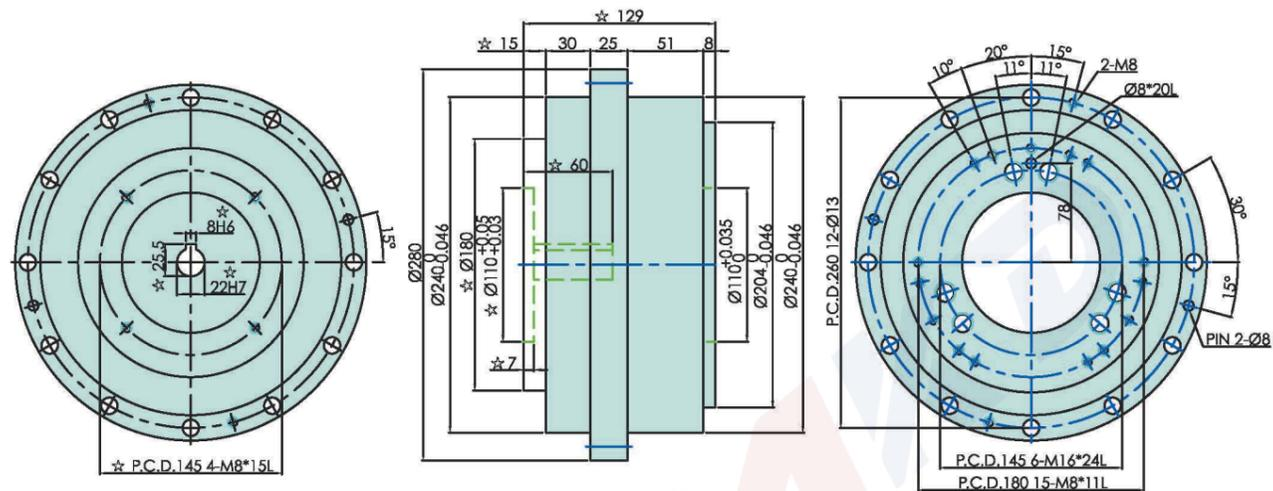
1. "☆"The dimensions modify with motor specification.
