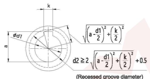
Set the diameter of the recessed groove (d2) so that it is larger than the corner of the keyway
