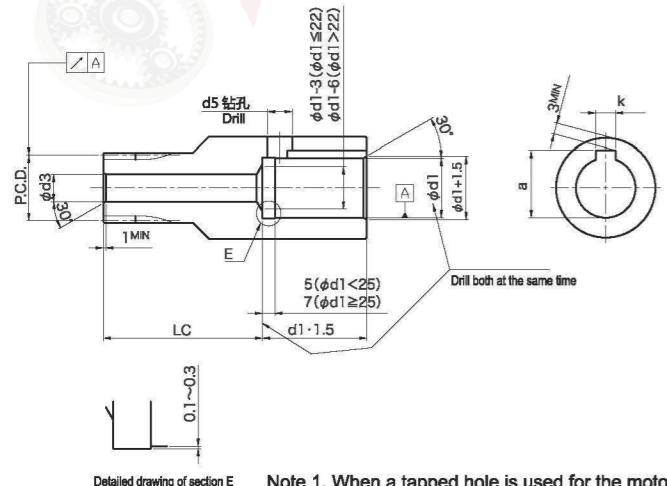
Applicable motor shaft diameters for standard input gear ( mm)
