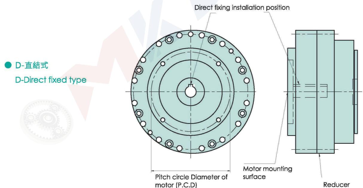
1. Place motor shaft key and reducer input shaft key way in a straight line, and insert motor shaft into reducer input shaft.
